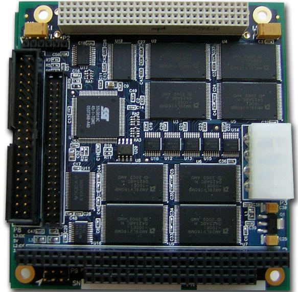
FlashDrive/104 is a flash based, solid state storage module designed using the latest NAND technology. This rugged storage module is a robust, drop-in replacement for magnetic hard drives that can be prone to mechanical failures or corruption due to shock and vibration.
